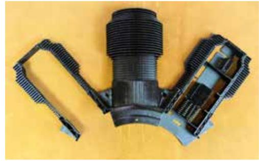
*Left: One half, 3D printed, cylinder head.
